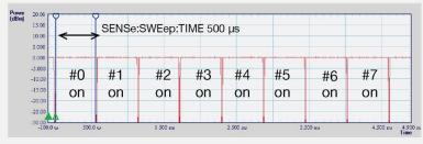
SENS:MRATE FAST TRIG:COUN 100 TRIG:SOUR EXT SENS:SWE:APER 500 µs TRIG:DEL 50 µs \*OPC? FETC? //Read back time-selectivity average power with an array of 100 data
