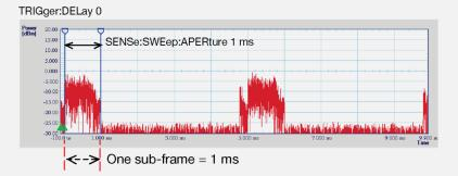
SENS:MRATE FAST TRIG:COUN 100 TRIG:SOUR EXT SENS:SWE:APER 1 ms TRIG:DEL 0 \*OPC? FETC? //Read back the burst average power with an array of 100 data
