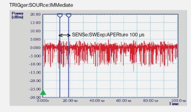
To obtain real time measurement of 10,000 readings per second, set the following: CAL:AUTO OFF //optional setting SENS:AVER:COUN 1 //optional setting SENS:AVER:SDET OFF //optional setting TRIG:DEL:AUTO OFF //optional setting UNIT:POW W //optional setting FORM REAL SENS:MRATE FAST TRIG:COUN 100 SENS:SOUR IMM SENS:SWE:APER 100 µs TRIG:DEL 0 \*OPC? FETC? //Read back the waveform average power with an array of 100 data
