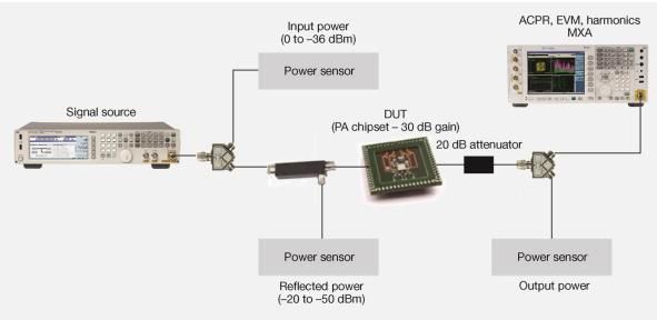
Figure 1. Typical test setup for wireless chipset manufacturing test
